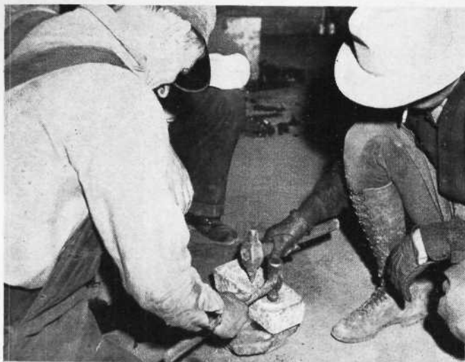
5—These industrious men are hammering a gold brick to free it from particles of Silver , Sand , Glass .
