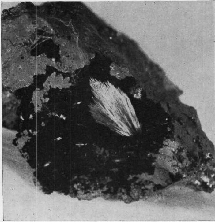
Magnified picture of the lacy crystals of brochantite as they occur in vugs in the rock matrix.
